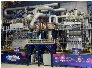
RTX-8 / RTX-7 (new): GTC Shanghai CN 4 cyl, 52 cm bore Methanol, ammonia / Gas LP-DF
