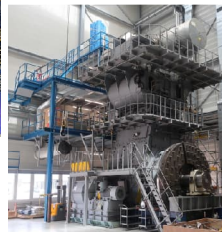
SCE (brand new): ERIC CH 1 cyl, 50 cm bore All fuels / concepts
