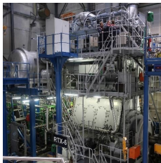
RTX-6 (existing): ERIC CH 4 cyl, 50 cm bore Diesel, methanol
